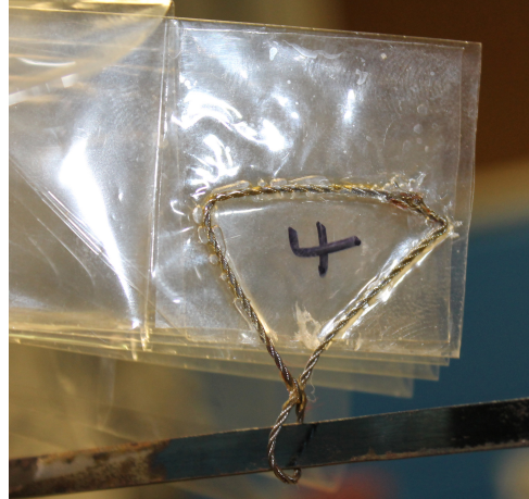
Fig. 6. Encapsulated attachment of the wire loop in the corner of the sail
