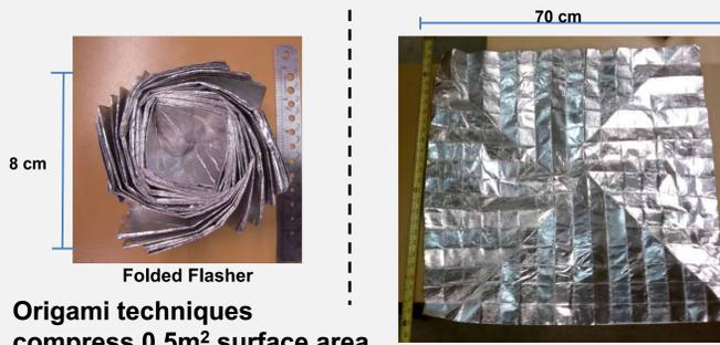
Origami techniques compress 0.5m<sup>2</sup> surface area flasher into a 0.5U payload volume.
