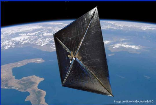
Deploying a differential drag surface to alter relative velocity and position of the satellite.
